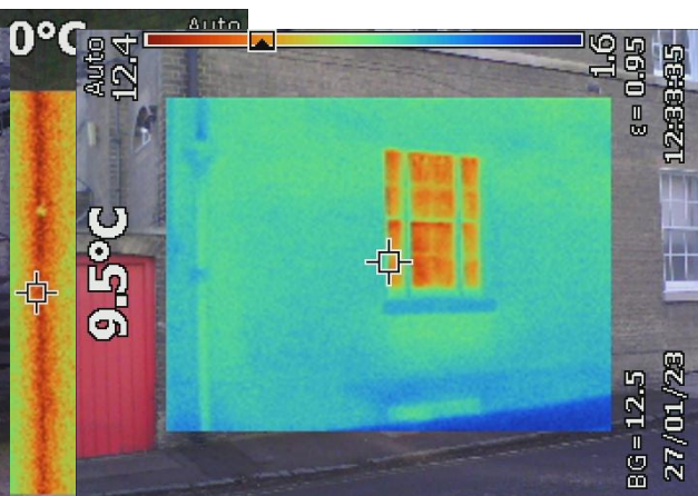
This image shows heat escaping from window but also a warm spot under the window where a draught is present.
