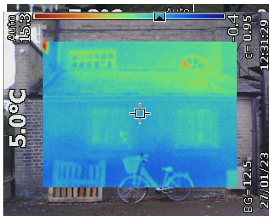
This image shows heat loss through the roof and around the bay structure around the ground floor meeting room. Here heat can be seen leaking at the junctions of the building's wall with the
