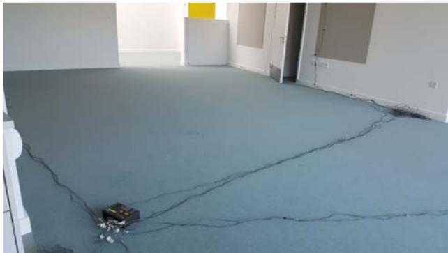
**Process/methodology:** The project involves setting up thermistors, thermocouples and data loggers to measure U-values and to capture the temperature distributions of the classroom caused by ventilation changes or by underfloor heating.
